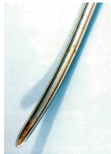
Figure B.3 - Organic residues that have become brown and encrusted
