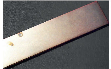
Figure B.4 - Enlarged cross-section of pitting corrosion Figure B.5 - Pitting corrosion on a chisel
