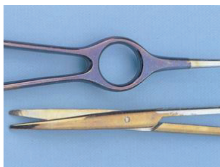
Figure B.2 - Discoloration caused by silicates
